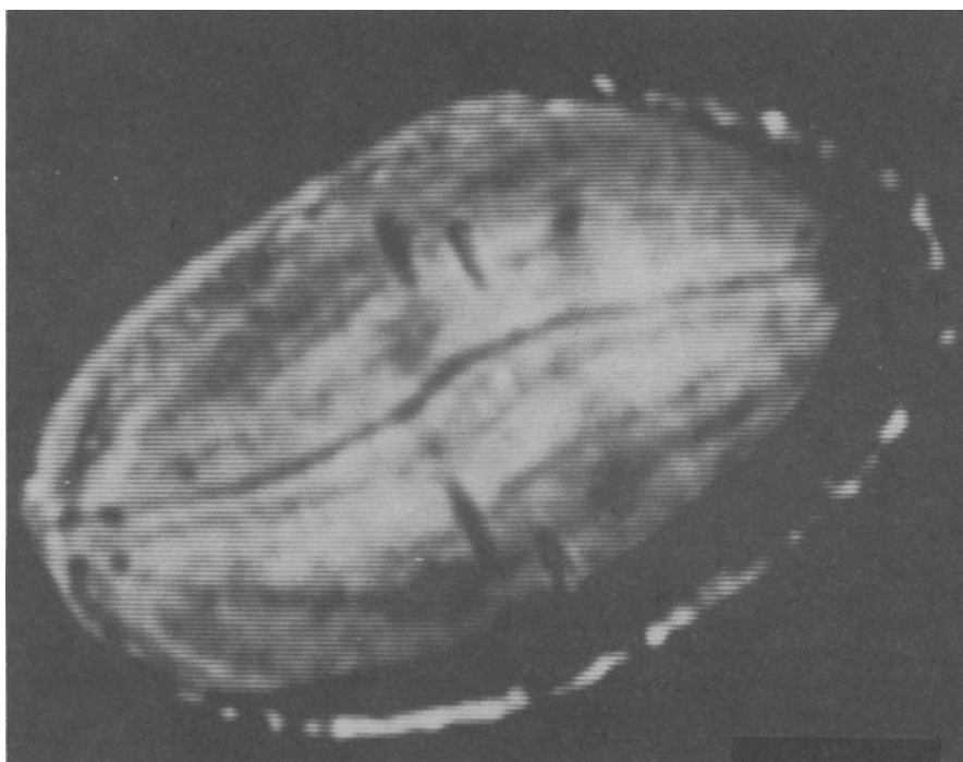
FIG. 1. NMR \mu -image of a 0.5-mm horizontal cross section of a sunflower seed at 400 MHz.
